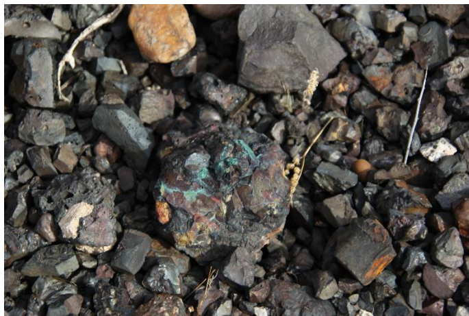
Copper Slag with Green Oxidation
