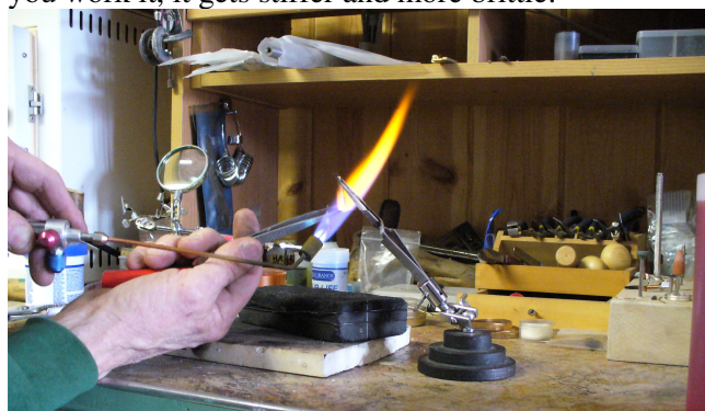
[ Annealing the gold wire by heating with a torch ]
