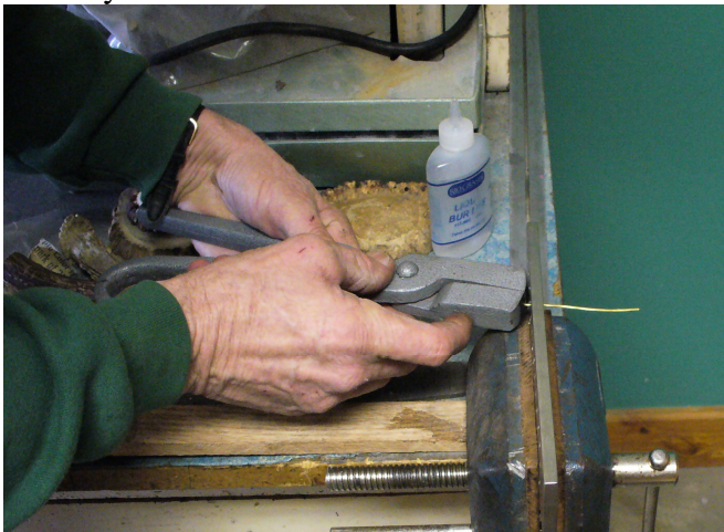
[Drawing wire through the draw plate with tongs]
