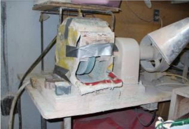
Start working off the corners on a flat sides wheel of a 100 grit carborundum grinding wheel. When the cube has been rounded down, he moves to the middle of a wheel that has a round channel worn into the middle. (Keith used hard agate and metal to wear the round groove into the wheel.) Pushing the emerging marble into the groove, rotate it to eliminate all the high spots. Check for them with a round
