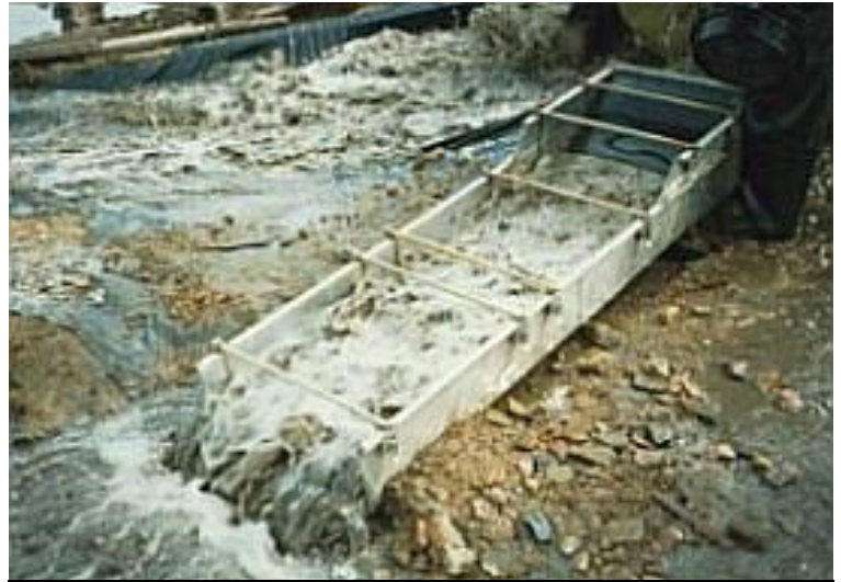
Mining placer box replicates the action of natural placer deposits.
